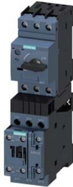
Fuseless motor starter Direct start 600VAC Size S0 1.8-2.5A 24V DC screw connection For screw mounting Or 35 mm rail-mounting Type of coordination 2 IQ = 150 KA Also full fills type Of coordination 1 1NO+1NC (contactor)
