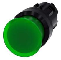
Illuminated mushroom pushbutton, 22 mm, round, plastic, green, 30 mm, momentary contact type, with laser labeling, upper case and lower case, always upper case at beginning of line
