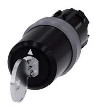
key-operated switch Siemens, 22 mm, round, plastic with metal front ring, lock number SSG10, with 2 keys, 3 switch positions I>O<II, momentary contact on the left, latching on the right, actuating angle 2x45°, 10:30h/12h/13:30h, key removal O+II, with laser labeling, upper case and lower case, always upper case at the beginning of the word
