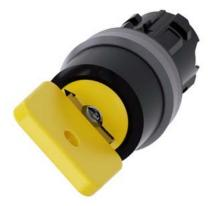
Key-operated switch O.M.R, 22 mm, round, plastic with metal front ring, lock number 73033, yellow, with 2 keys, 2 switch positions O<I, momentary contact type, Actuating angle 45°, 10:30h/12h, key removal O, with laser labeling, upper case and lower case, always upper case at beginning of line
