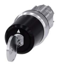
Key-operated switch BKS, 22 mm, round, metal, shiny, special lock, with 2 keys, 3 switch positions I-O<II, latching on the left, momentary contact type on the right, actuating angle 2x45°, 10:30h/12h/13:30h, key removal O, Note: BKS locking systems E1 - E25 supplied without key
