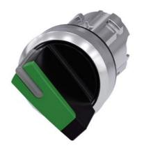
Selector switch, illuminable, 22 mm, round, metal, shiny, green, selector switch, short, 2 switch positions O<I, momentary contact type, Actuating angle 45°, 10:30h/12h, Z=50-unit packaging
