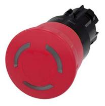
EMERGENCY STOP mushroom pushbutton, illuminable, 22 mm, round, plastic, red, 40 mm, positive latching, acc. to EN ISO 13850, rotate-to-unlatch, with laser labeling, inscription or symbol Customer-specific selection with SIRIUS ACT configurator (CIN)
