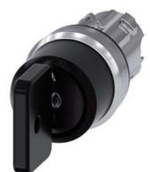
Key-operated switch O.M.R, 22 mm, round, metal, shiny, lock number 73034, black, with 2 keys, 3 switch positions I>O<II, momentary contact type, actuating angle 2x45°, 10:30h/12h/13:30h, key removal O, with laser labeling, upper case and lower case, always upper case at beginning of line
