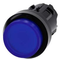
Illuminated pushbutton, 22 mm, round, plastic, blue, pushbutton, raised momentary contact type, with laser labeling, symbol number according to, ISO 7000 or IEC 60417
