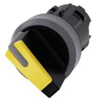
Selector switch, illuminable, 22 mm, round, plastic with metal front ring, yellow, selector switch, short, 2 switch positions O-I, latching, actuating angle 90°, 10:30h/13:30h, Z=50-unit packaging
