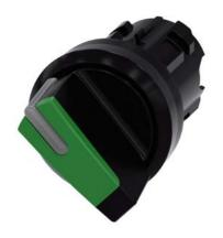
Selector switch, illuminable, 22 mm, round, plastic, green, selector switch, short, 2 switch positions O-I, latching, actuating angle  $90^\circ$ , 10:30h/13:30h, with laser labeling, inscription or symbol Customer-specific selection with SIRIUS ACT configurator (CIN)
