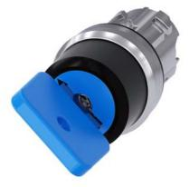
Key-operated switch O.M.R, 22 mm, round, metal, shiny, lock number 73038, blue, with 2 keys, 2 switch positions O-I, latching, actuating angle 90°, 10:30h/13:30h, key removal I, with laser labeling, upper case and lower case, always upper case at the beginning of the word
