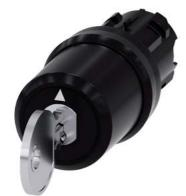
key-operated switch Siemens, 22 mm, round, plastic, lock number SSG10, with 2 keys, 3 switch positions I>O<II, momentary contact on the left, latching on the right, actuating angle 2x45°, 10:30h/12h/13:30h, key removal II Z=50-unit packaging
