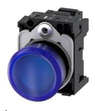
Indicator lights, 22 mm, round, plastic, blue, lens, smooth, with holder, LED module, with integrated LED 24 V AC/DC, spring-type terminal, with laser labeling, upper case and lower case, always upper case at the beginning of the word
