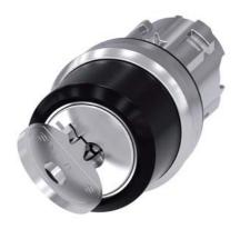
RONIS key-operated switch, 22 mm, round, metal, shiny, lock number SB30, with 2 keys, 2 switch positions O-I, latching, actuating angle 90°, 10:30h/13:30h, key removal O, possible special locks: SB31, 421, 455, with laser labeling, upper case and lower case, always upper case at beginning of line
