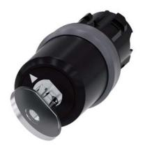
Key-operated switch BKS, 22 mm, round, plastic with metal front ring, Lock number E1 (VW), without key, 2 switch positions O-I, latching, actuating angle 90°, 10:30h/13:30h, key removal O+I, with laser labeling, upper case and lower case, always upper case at the beginning of the word
