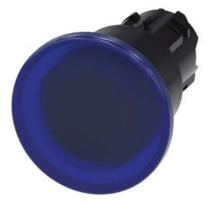
Illuminated mushroom pushbutton, 22 mm, round, plastic, blue, 40mm, latching, pull-to-unlatch mechanism, with laser labeling, upper case and lower case, always upper case at beginning of line
