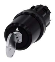
key-operated switch Siemens, 22 mm, round, plastic, lock number SSG10, with 2 keys, 3 switch positions I>O<II, momentary contact on the left, latching on the right, actuating angle  $2x45^{\circ}$ , 10:30h/12h/13:30h, key removal O, with laser labeling, upper case and lower case, always upper case at the beginning of the word
