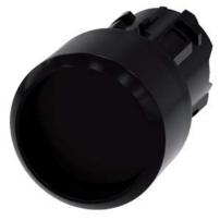
Pushbutton, 22 mm, round, plastic, black, Front ring, raised momentary contact type, with laser labeling, inscription or symbol Customer-specific selection with SIRIUS ACT configurator (CIN)
