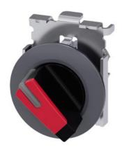
Selector switch, illuminable, 30 mm, round, Metal, matte, red, selector switch, short, front ring for flush installation, 2 switch positions O-I, latching, actuating angle 90°, 10:30h/13:30h, with laser labeling, inscription or symbol Customer-specific selection with SIRIUS ACT configurator (CIN)
