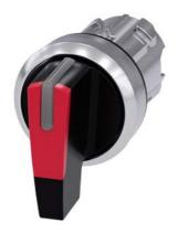
Selector switch, illuminable, 22 mm, round, metal, shiny, red, selector switch, long, 3 switch positions I>O<II, momentary contact on the left, latching on the right, actuating angle 2x45°, 10:30h/12h/13:30h, Z=50-unit packaging
