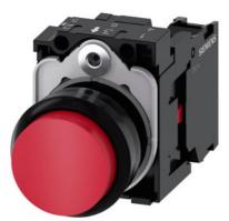
Pushbutton, 22 mm, round, plastic, red, pushbutton, raised, momentary contact type, with holder 1 NC, screw terminal, with laser labeling, inscription or symbol Customer-specific selection with SIRIUS ACT configurator (CIN)
