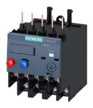
Overload relay 1.8...2.5 A Thermal For motor protection Size S00, Class 10 Contactor mounting Main circuit: Ring cable lug Auxiliary circuit: ring cable lug Manual-Automatic-Reset
