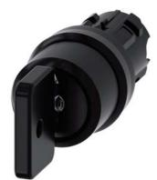
Key-operated switch O.M.R, 22 mm, round, plastic, lock number 73034, black, with 2 keys, 3 switch positions I-O-II, latching, actuating angle 2x45°, 10:30h/12h/13:30h, key removal O, with laser labeling, upper case and lower case, always upper case at beginning of line
