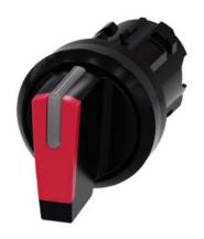
Selector switch, illuminable, 22 mm, round, plastic, red, selector switch, short, 3 switch positions I-O<II, left latching, right momentary contact type, actuating angle 2x45°, 10:30h/12h/13:30h, with laser labeling, inscription or symbol Customer-specific selection with SIRIUS ACT configurator (CIN)
