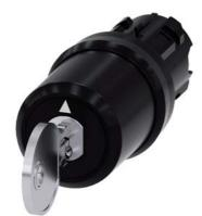
Key-operated switch BKS, 22 mm, round, plastic, lock number S1, with 2 keys, 3 switch positions I-O-II, latching, actuating angle 2x45°, 10:30h/12h/13:30h, Key removal I+O+II, with laser labeling, inscription or symbol Customer-specific selection with SIRIUS ACT configurator (CIN)
