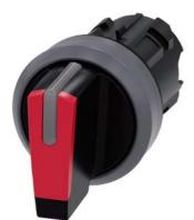
Selector switch, illuminable, 22 mm, round, plastic with metal front ring, red, selector switch, short, 3 switch positions I>O<II, momentary contact type, actuating angle 2x45°, 10:30h/12h/13:30h, with laser labeling, upper case and lower case, always upper case at beginning of line
