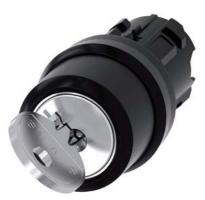
RONIS key-operated switch, 22 mm, round, plastic, lock number 455, with 2 keys, 2 switch positions O<I, momentary contact type, Actuating angle 45°, 10:30h/12h, key removal O, with laser labeling, inscription or symbol Customer-specific selection with SIRIUS ACT configurator (CIN)
