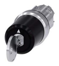
key-operated switch Siemens, 22 mm, round, metal, shiny, special lock, with 2 keys, 3 switch positions I>O<II, momentary contact on the left, latching on the right, actuating angle  $2x45^{\circ}$ , 10:30h/12h/13:30h, key removal O
