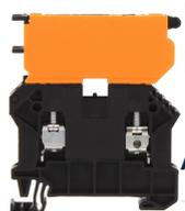
Fuse-disconnect terminal, Screw connection, Mounting type: Mounting rail TS 35/7.5, Rated cross-section: 6 mm<sup>2</sup>, Width: 8.1 mm, Colour: Black
