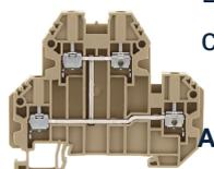
Double-level terminal, Screw connection, Mounting type: Mounting rail TS 35/7.5, Rated cross-section: 2.5 mm<sup>2</sup>, Width: 5.1 mm, Colour: Beige
