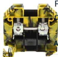
Feed-through terminal, Screw connection, Mounting type: Mounting rail TS 35/7.5, Rated cross-section: 16 mm<sup>2</sup>, Width: 12.1 mm, Colour: Black-yellow
