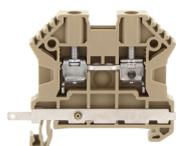
Feed-through terminal, Screw connection, Mounting type: Mounting rail TS 35/7.5, Rated cross-section: 4 mm<sup>2</sup>, Width: 6 mm, Colour: Beige
