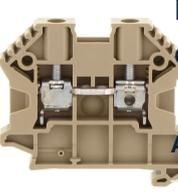
Feed-through terminal, Screw connection, Mounting type: Mounting rail TS 35/7.5, Rated cross-section: 2.5 mm<sup>2</sup>, Width: 5 mm, Colour: Beige
