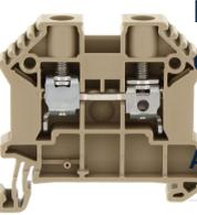
Feed-through terminal, Screw connection, Mounting type: Mounting rail TS 35/7.5, Rated cross-section: 10 mm<sup>2</sup>, Width: 8 mm, Colour: Beige
