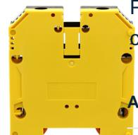
Feed-through terminal, Screw connection, Mounting type: Mounting rail TS 35/7.5, Rated cross-section: 70 mm<sup>2</sup>, Width: 20.5 mm, Colour: Black-yellow
