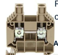
Feed-through terminal, Screw connection, Mounting type: Mounting rail TS 35/7.5, Rated cross-section: 16 mm<sup>2</sup>, Width: 12.1 mm, Colour: Beige
