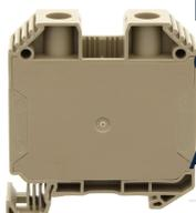
Feed-through terminal, Screw connection, Mounting type: Mounting rail TS 35/7.5, Rated cross-section: 35 mm<sup>2</sup>, Width: 16.1 mm, Colour: Beige
