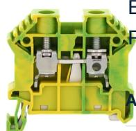
EX-Protective earth terminal, Screw connection, Mounting type: Mounting rail TS 35/7.5, Rated cross-section: 16 mm<sup>2</sup>, Width: 10 mm, Colour: Green-yellow
