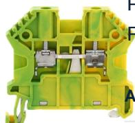
Protective earth terminal, Screw connection, Mounting type: Mounting rail TS 35/7.5, Rated cross-section: 2.5 mm<sup>2</sup>, Width: 5 mm, Colour: Green-yellow
