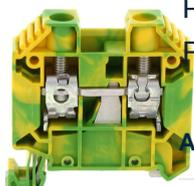
Protective earth terminal, Screw connection, Mounting type: Mounting rail TS 35/7.5, Rated cross-section: 16 mm<sup>2</sup>, Width: 12.1 mm, Colour: Green-yellow
