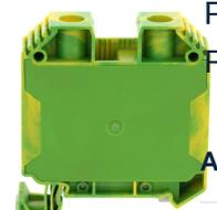
Protective earth terminal, Screw connection, Mounting type: Mounting rail TS 35/7.5, Rated cross-section: 35 mm<sup>2</sup>, Width: 16.1 mm, Colour: Green-yellow
