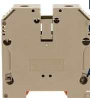
Feed-through terminal, Screw connection, Mounting type: Mounting rail TS 35/7.5, Rated cross-section: 70 mm<sup>2</sup>, Width: 20.5 mm, Colour: Beige
