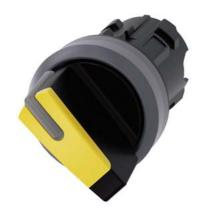
Selector switch, illuminable, 22 mm, round, plastic with metal front ring, yellow, selector switch, short, 2 switch positions O<I, momentary contact type, Actuating angle 45°, 10:30h/12h, with laser labeling, lower case
