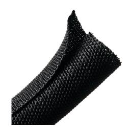
Center-slit overlapping design allows quick and easy access to the wires and cables for future maintenance or inspection without disassembly. Flexible material allows it to easily wrap around a variety of component shapes and sizes, making it easier to use than slit-loom tubing or spiral-wrap materials.
