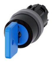
Key-operated switch O.M.R, 22 mm, round, plastic with metal front ring, lock number 73038, blue, with 2 keys, 3 switch positions I-O<II, left latching, right momentary contact type, actuating angle  $2x45^{\circ}$ , 10:30h/12h/13:30h, key removal O, with laser labeling, lower case
