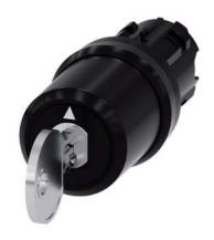
key-operated switch Siemens, 22 mm, round, plastic, lock number SSG10, with 2 keys, 3 switch positions I-O<II, left latching, momentary contact type on the right, actuating angle 2x45°, 10:30h/12h/13:30h, key removal O, with laser labeling, upper case and lower case, always upper case at beginning of line
