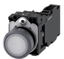
Illuminated pushbutton, 22 mm, round, plastic with metal front ring, white, pushbutton, flat, momentary contact type, with holder, 1 NO+1 NC, LED module with integrated LED 110 V AC, screw terminal, with laser labeling, inscription or symbol Customer-specific selection with SIRIUS ACT configurator (CIN)
