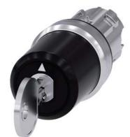
key-operated switch Siemens, 22 mm, round, metal, shiny, lock number SSG10, with 2 keys, 3 switch positions I-O-II, latching, actuating angle 2x45°, 10:30h/12h/13:30h, key removal I+O+II, with laser labeling, inscription or symbol customer-specific selection with SIRIUS ACT configurator (CIN)
