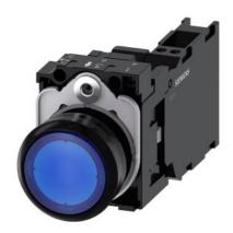
Illuminated pushbutton, 22 mm, round, plastic, blue, pushbutton, flat, momentary contact type, with holder, 1 NO+1 NC, LED module with integrated LED 110 V AC, spring-type terminal, with laser labeling, symbol number according to, ISO 7000 or IEC 60417
