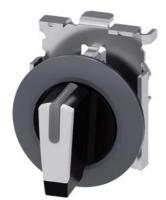
Selector switch, illuminable, 30 mm, round, Metal, matte, white, selector switch, short, front ring for flush installation, 3 switch positions I-O-II, latching, actuating angle  $2x45^{\circ}$ , 10:30h/12h/13:30h, with laser labeling, upper case and lower case, always upper case at the beginning of the word
