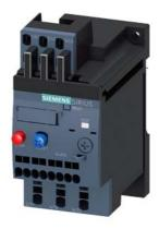
Overload relay 11...16 A Thermal For motor protection Size S00, Class 10 Stand-alone installation Main circuit: Spring-type terminal Auxiliary circuit: spring-type terminal Manual-Automatic-Reset
