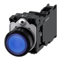
Illuminated pushbutton, 22 mm, round, plastic, blue, pushbutton, flat, momentary contact type, with holder, 1 NO+1 NC, LED module with integrated LED 110 V AC, Spring-type terminal
