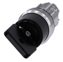
Key-operated switch O.M.R, 22 mm, round, metal, shiny, lock number 73034, black, with 2 keys, 2 switch positions O-I, latching, actuating angle 90°, 10:30h/13:30h, key removal O+I, with laser labeling, upper case and lower case, always upper case at the beginning of the word
