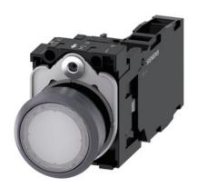
Illuminated pushbutton, 22 mm, round, plastic with metal front ring, white, pushbutton, flat, momentary contact type, with holder, 1 NO+1 NC, LED module with integrated LED 24 V AC/DC, screw terminal, with laser labeling, upper case
