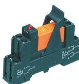
Pre-assembled relay module PRS..., Screw connection, Consisting of: relay socket base, power contact relay, pluggable display/suppression module and holding clip, 2 CO contacts, Input voltage: 60 VDC
