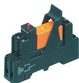
Pre-assembled relay module PRS..., Screw connection, Consisting of: relay socket base, power contact relay, pluggable display/suppression module and holding clip, 1 CO contact, Input voltage: 60 VDC
