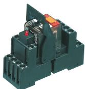
Pre-assembled relay module PRS..., Screw connection, Consisting of: relay socket base, power contact relay, pluggable display/suppression module and holding clip, 4 CO contacts, Input voltage: 60 VDC
