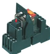
Pre-assembled relay module PRS..., Screw connection, Consisting of: relay socket base, power contact relay, pluggable display/suppression module and holding clip, 4 CO contacts, Input voltage: 110 VDC
