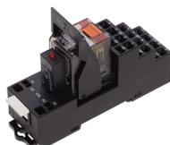
Pre-assembled relay module PRS..., Tension-spring connection, Consisting of: relay socket base, power contact relay, pluggable display/suppression module and holding clip, 4 CO contact, Input voltage: 60 VDC
