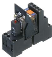
Pre-assembled relay module PRS..., Screw connection, Consisting of: relay socket base, power contact relay, pluggable display/suppression module and holding clip, 4 CO contacts, Input voltage: 60 VDC
