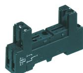
Relay socket base PRS, for miniature power relay with 1 CO contact, Screw connection, Plug-in option for input/suppression modules, Mounting type: Mounting rail TS 35
