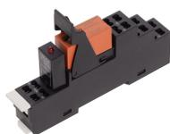
Pre-assembled relay module PRS..., Tension-spring connection, Consisting of: relay socket base, power contact relay, pluggable display/suppression module and holding clip, 2 CO contact, Input voltage: 48 VDC
