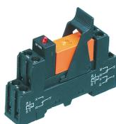
Pre-assembled relay module PRS..., Screw connection, Consisting of: relay socket base, power contact relay, pluggable display/suppression module and holding clip, 2 CO contacts, Input voltage: 24 VAC
