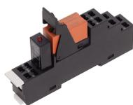
Pre-assembled relay module PRS..., Tension-spring connection, Consisting of: relay socket base, power contact relay, pluggable display/suppression module and holding clip, 2 CO contact, Input voltage: 60 VDC
