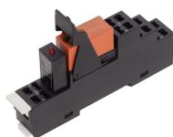
Pre-assembled relay module PRS..., Tension-spring connection, Consisting of: relay socket base, power contact relay, pluggable display/suppression module and holding clip, 2 CO contact, Input voltage: 48 VAC
