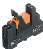
Pre-assembled relay module PRS..., Screw connection, Consisting of: relay socket base, power contact relay, pluggable display/suppression module and holding clip, 2 CO contacts, Input voltage: 48 VDC
