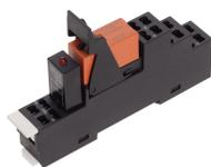
Pre-assembled relay module PRS..., Tension-spring connection, Consisting of: relay socket base, power contact relay, pluggable display/suppression module and holding clip, 2 CO contact, Input voltage: 230 VAC
