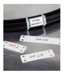
Identification Marker Plates can be marked with a permanent pen, printed labels or hot stamped for a wide variety of labeling options. Any size bundle diameter can be marked because it is only dependent upon the length of the cable tie selected, provided the cable tie width does not exceed .29".
