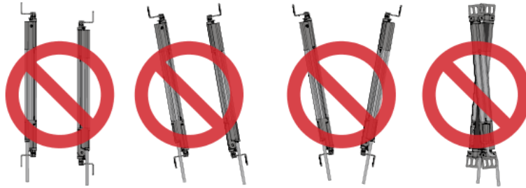
Figure 18. Incorrect Sensor Alignment
