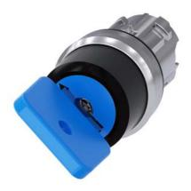
Key-operated switch O.M.R, 22 mm, round, metal, shiny, lock number 73038, blue, with 2 keys, 2 switch positions O<I, momentary contact type, Actuating angle 45°, 10:30h/12h, key removal O, with laser labeling, upper case and lower case, always upper case at the beginning of the word
