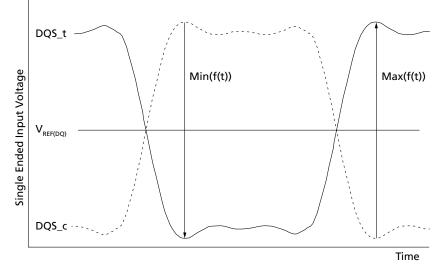
Note: 1.  $V_{REF(DQ)}$  is device internal setting value by  $V_{REF}$  training.
