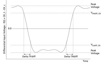
Notes: 1. Differential signal rising edge from V<sub>ILdiff\_DQS</sub> to V<sub>IHdiff\_DQS</sub> must be monotonic slope.
