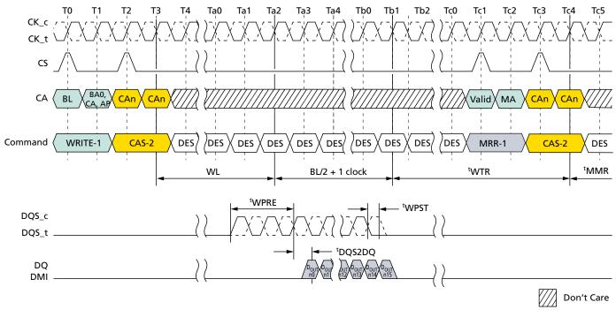
Notes: 1. Write BL = 16, Write postamble = 0.5nCK, DQ/DQS:  $V_{SSQ}$  termination.
