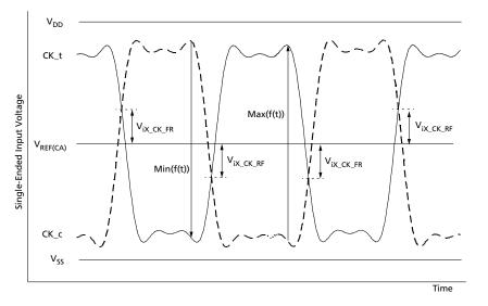
Note: 1. The base levels of  $V_{ix\_CK\_FR}$  and  $V_{ix\_CK\_RF}$  are  $V_{REF(CA)}$  that is device internal setting value by  $V_{REF}$  training.
