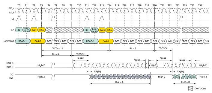
Figure 119: Consecutive READ: <sup>t</sup>CCD = MIN + 3, Preamble = Toggle, 0.5*n*CK Postamble
