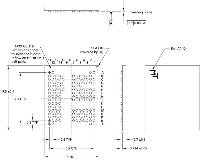
Notes: 1. All dimensions are in millimeters.2. Package height does not include room temperature warpage.
