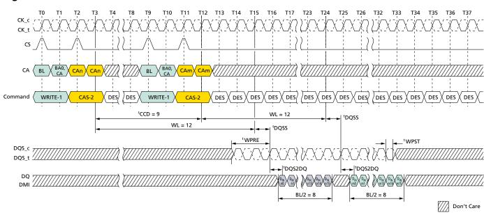
Figure 125: Consecutive WRITE: <sup>t</sup>CCD = MIN + 1, 0.5*n*CK Postamble
