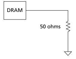
Note: 1. All output timing parameter values are reported with respect to this reference load; this reference load is also used to report slew rate.
