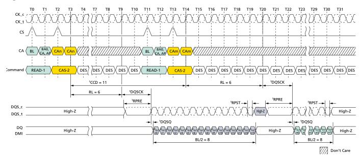
Figure 121: Consecutive READ: <sup>t</sup>CCD = MIN + 3, Preamble = Static, 0.5*n*CK Postamble
