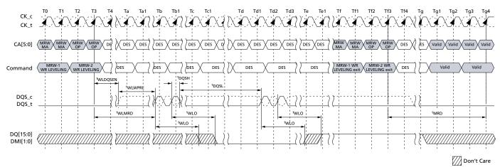
Note: 1. Clock can be stopped except during DQS toggle period (CK\_t = LOW, CK\_c = HIGH). However, a stable clock prior to sampling is required to ensure timing accuracy.
