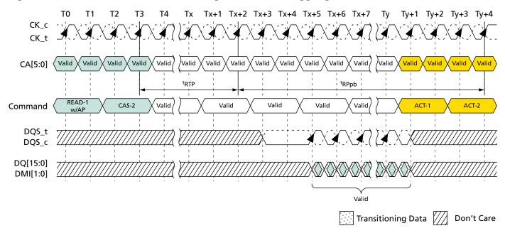
Figure 136: Burst READ With Auto Precharge – BL32, Toggling Preamble, 1.5nCK Postamble
