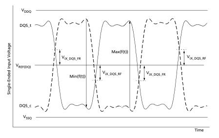
Note: 1. The base levels of  $V_{ix_DQS_FR}$  and  $V_{ix_DQS_RF}$  are  $V_{REF(DQ)}$  that is device internal setting value by  $V_{REF}$  training.
