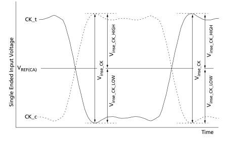
Note: 1.  $V_{REF(CA)}$  is device internal setting value by  $V_{REF}$  training.
