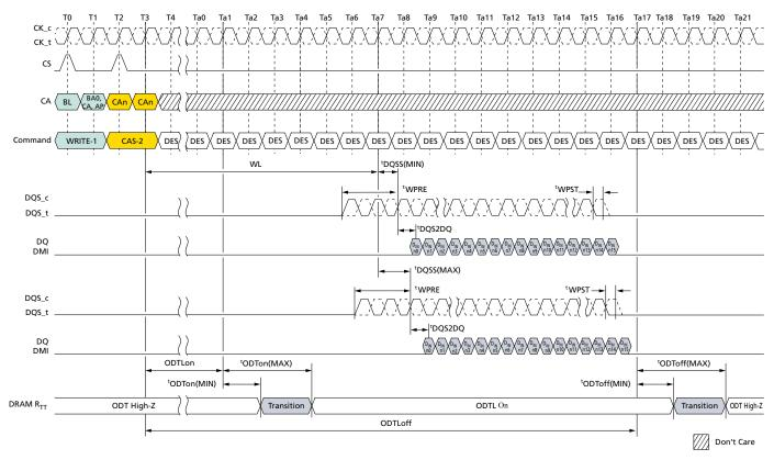
Notes: 1. BL = 16, Write postamble = 0.5nCK, DQ/DQS: V<sub>SSQ</sub> termination. 2. D<sub>IN</sub> n = data-in to column n.
