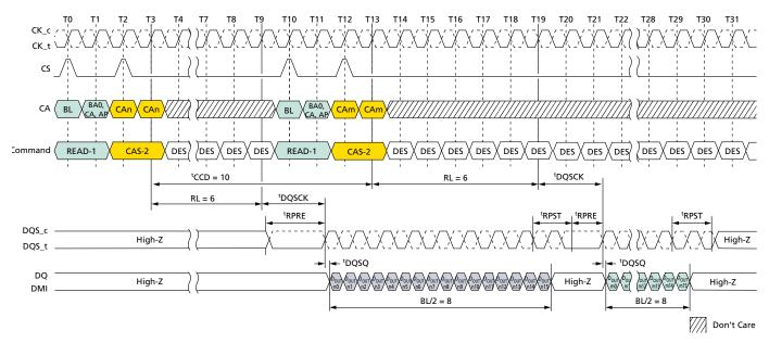
Notes: 1. BL = 16 for column *n* and column *m*; RL = 6; Preamble = Static; Postamble = 1.5nCK. 2. D<sub>OUT</sub> *n/m* = data-out from column *n* and column *m*.
