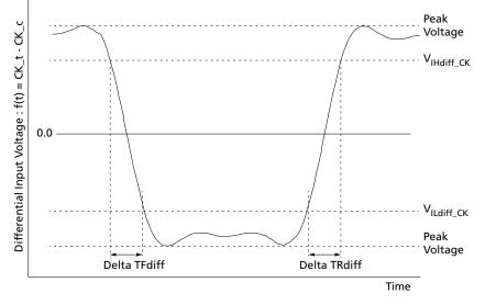
Notes: 1. Differential signal rising edge from V<sub>ILdiff\_CK</sub> to V<sub>IHdiff\_CK</sub> must be monotonic slope.
