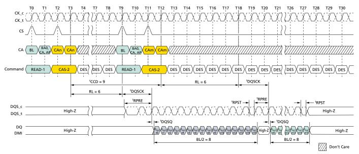
Notes: 1. BL = 16 for column *n* and column *m*; RL = 6; Preamble = Toggle; Postamble = 0.5nCK. 2. D<sub>OUT</sub> n/m = data-out from column *n* and column *m*.
