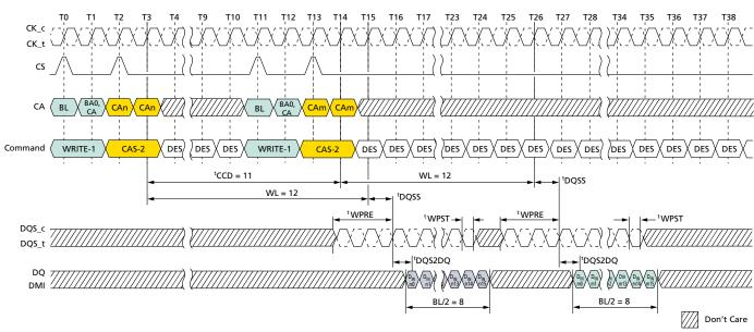
Figure 129: Consecutive WRITE: <sup>t</sup>CCD = MIN + 3, 0.5*n*CK Postamble
