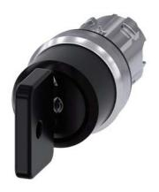
Key-operated switch O.M.R, 22 mm, round, metal, shiny, lock number 73034, black, with 2 keys, 3 switch positions I>O<II, momentary contact on the left, latching on the right, actuating angle 2x45°, 10:30h/12h/13:30h, Key removal II, with laser labeling, inscription or symbol Customer-specific selection with SIRIUS ACT configurator (CIN)
