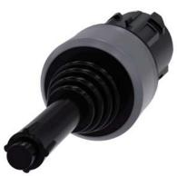
Coordinate switch, 22 mm, round, plastic with metal front ring, black, 4 switch positions, latching, with mechanical interlocking, with laser labeling, upper case
